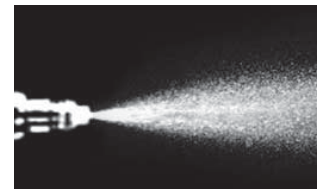
Injector spray pattern after P.i. treatment.
