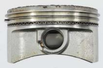
The piston and rings are virtually free of deposits and wear after 500 hours of severe-service testing in the Kawasaki\* FX 730 V engine.
